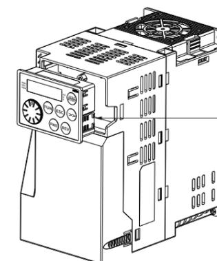
Press inwards on both sides to release the panel
